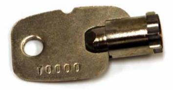
**Spaceguard Cylinder Lock Out Key**The lock out key is used with cylinder lock part 502705 to provide an overlock function. It does not open the lock. Overlocking prevents the regular key from working and is typically used by facility managers to block delinquent tenants from accessing their space.
